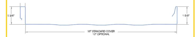
Flat panels are prone to excessive oil canning (visible waviness in the metal). *American Roofing Products does not recommend or warranty flat panels.*
